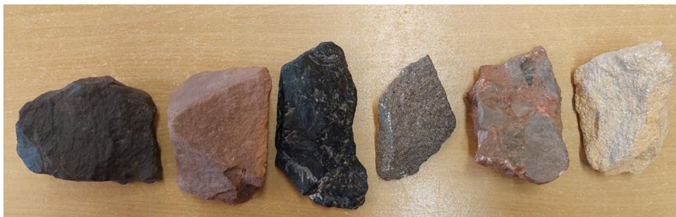
Above: samples from the Centre, from l to r: andesite, Old Red Sandstone, Black Rock Limestone, Valis Vale Limestone (overlies the BRL, blue on the right of the diagram), then the non-conformal Triassic conglomerate and the Inferior Oolite.
