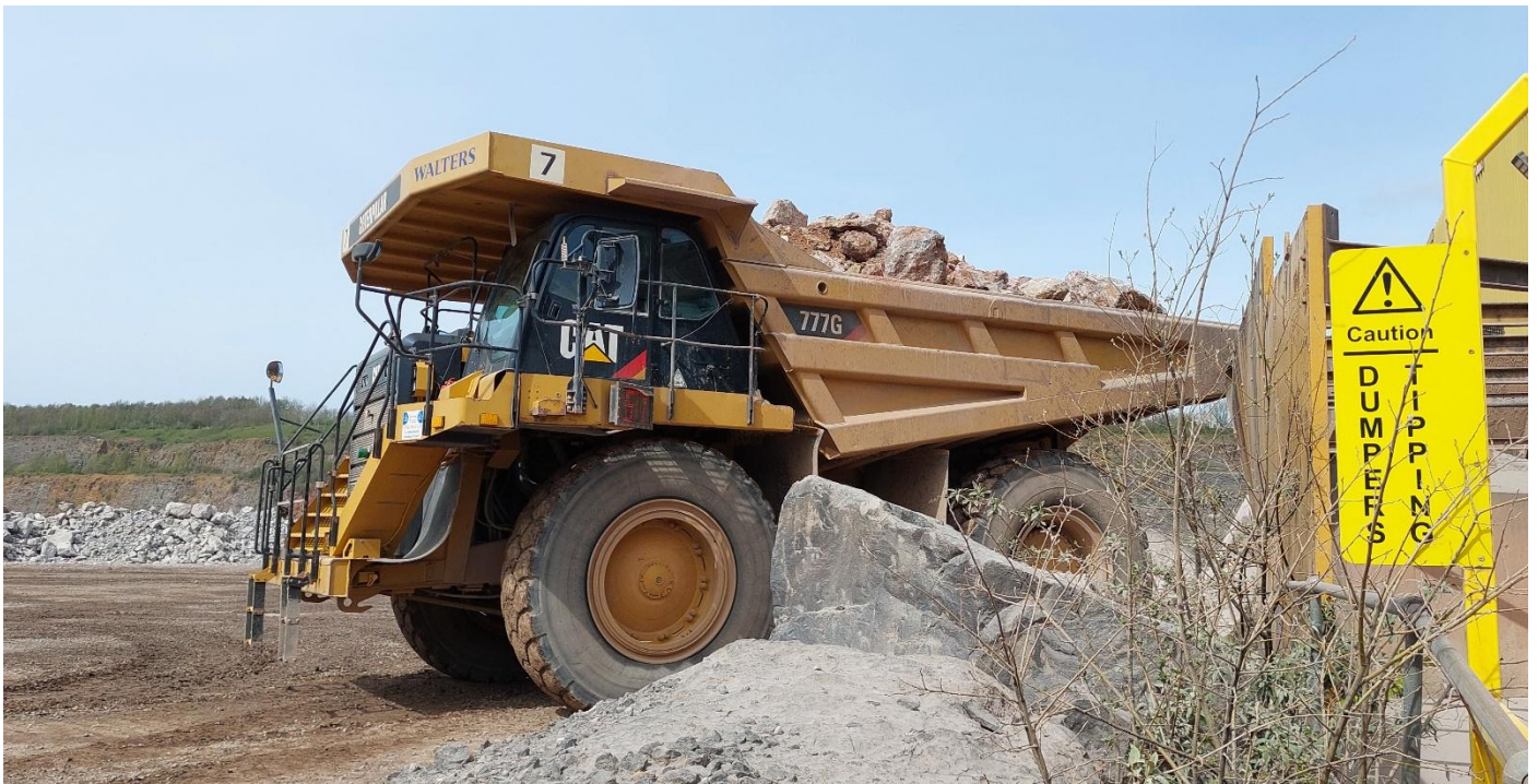
Above: the 6 million tons produced annually arrives at the primary crusher 100 tons at a time.
