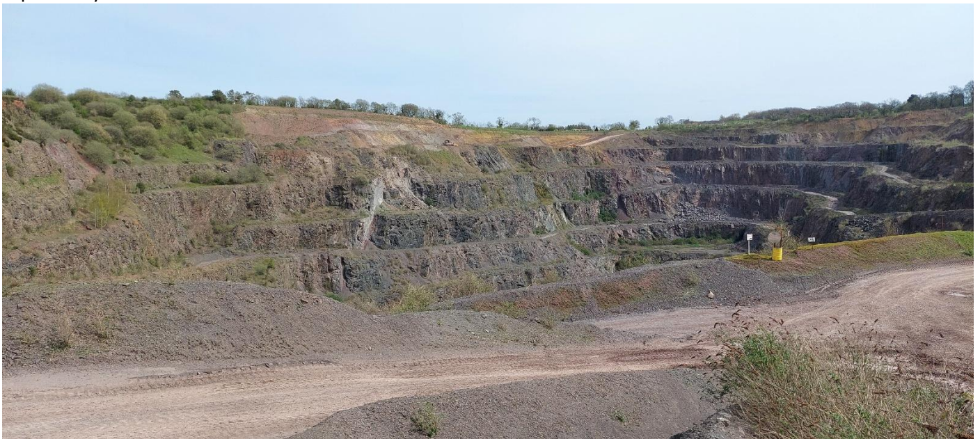
Above: Moon's Hill Quarry, where andesite is extracted. The red rock just left of centre in the picture is the Old Red Sandstone that overlies the igneous rock and separates it from the Black Rock Limestone extracted at Whatley.
